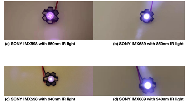
Figure 4: The detected IR lights (850nm and 940nm) on SONY IMX598 and IMX689
