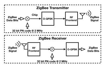
Figure 5: The ZigBee Transmitter and Receiver
