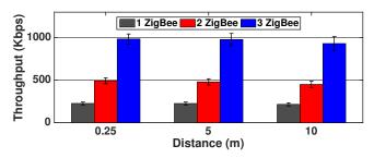
Figure 13: Backscatter to ZigBee throughput in Mobile Scenario. Passive-ZigBee has stable throughput over communication distance.
