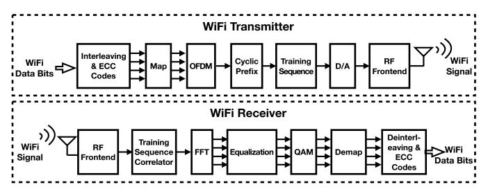
Figure 3: The WiFi Transmitter and Receiver
