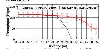
Figure 14: Backscatter to ZigBee Throughput under different Gateway Transmission Power
