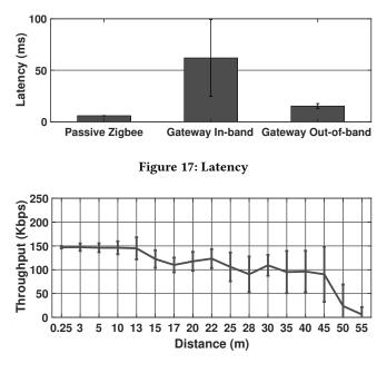
Figure 18: Throughput of Backscattering COTS WiFi to Zig-Bee in NLoS.
