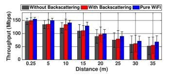
Figure 22: The impact to On-going WiFi Communications
