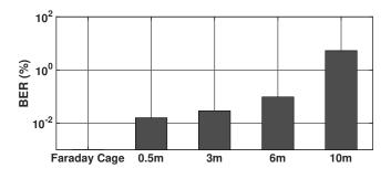
Figure 16: BER of Backscatter to ZigBee in NLoS
