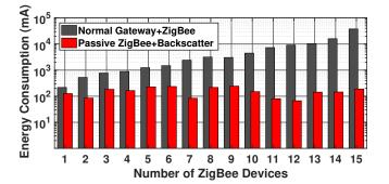
Figure 23: Energy Consumption (the y-axis is in log scale)
