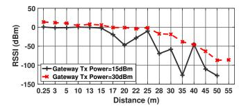
Figure 20: RSS @ ZigBee Receiver Side
