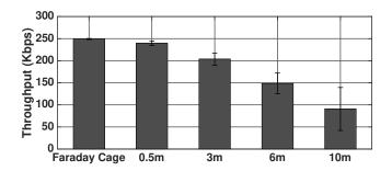
Figure 15: The throughput of Backscatter to ZigBee in NLoS
